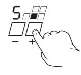
When pressing the plus-sensor the cooking zone starts at cooking setting 5, without boost.
